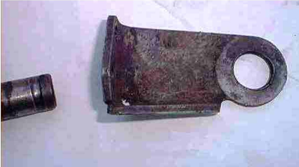
Pressure from shaft riding on the fixed mount has worn the mounting hole oblong
