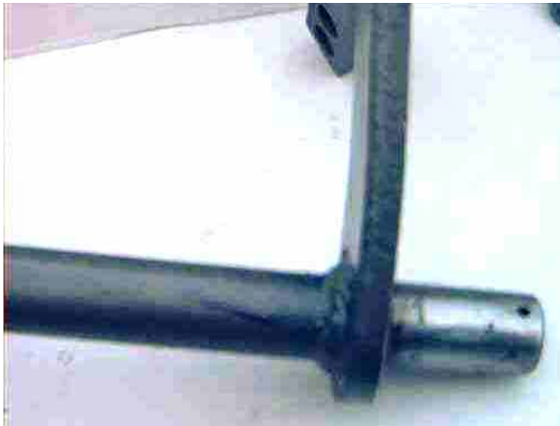
Cross shaft J2-25 repaired with weld and ground back to proper ID
