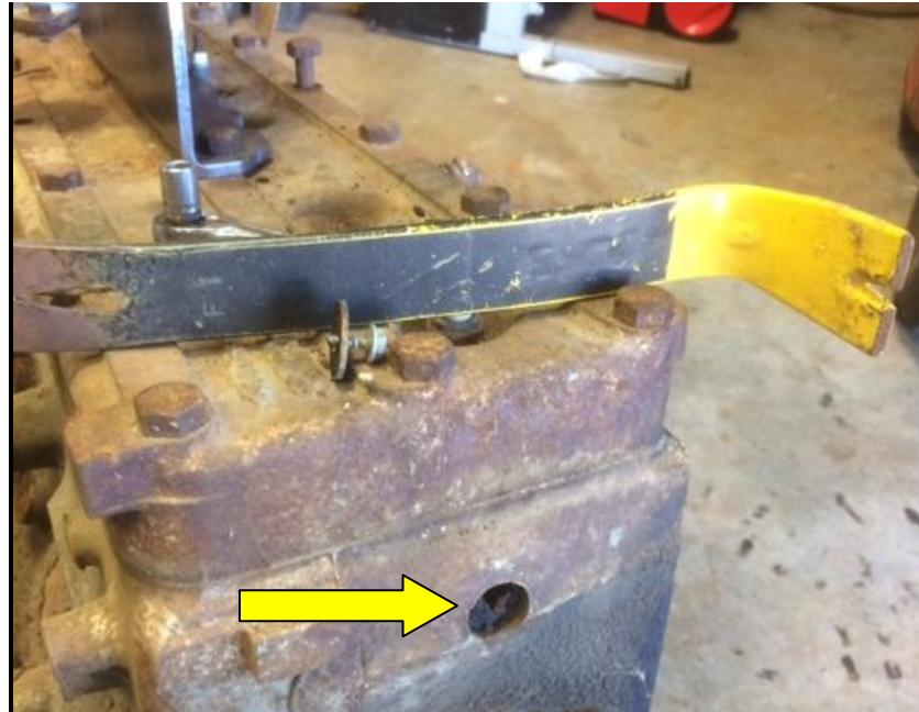
Step 3 -- Clamp a Vice Grip pliers to the tab end at water pump end of the water distribution tube.
