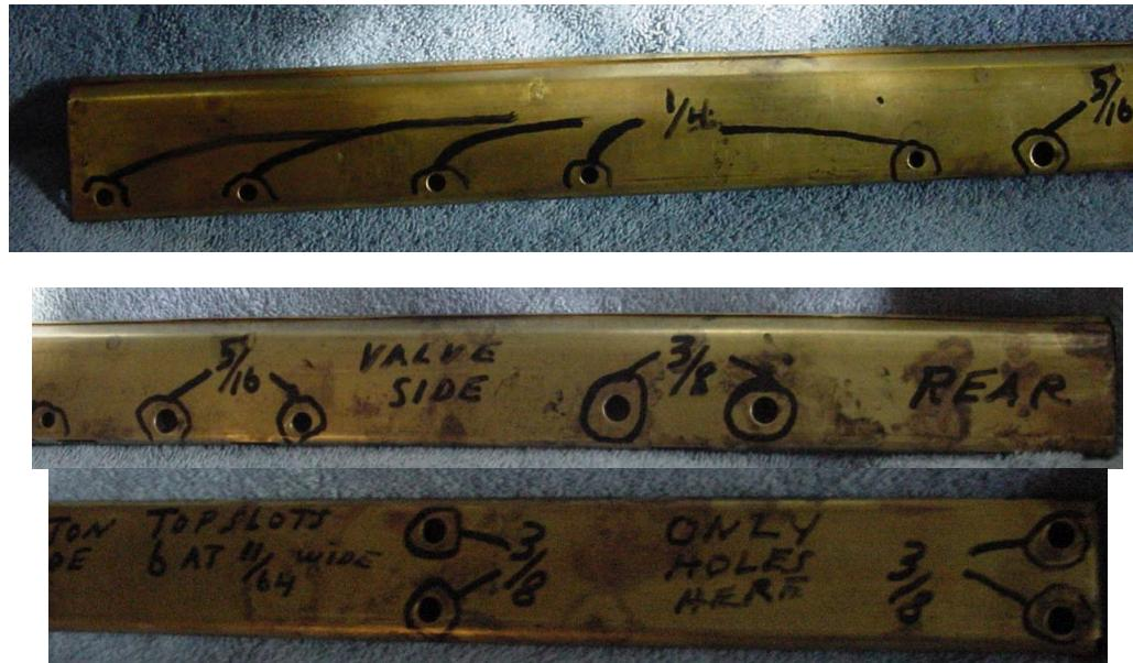
**1955-56 308 Deflector Manifold dimension's ( the early manifolds have less holes and some are smaller)**
