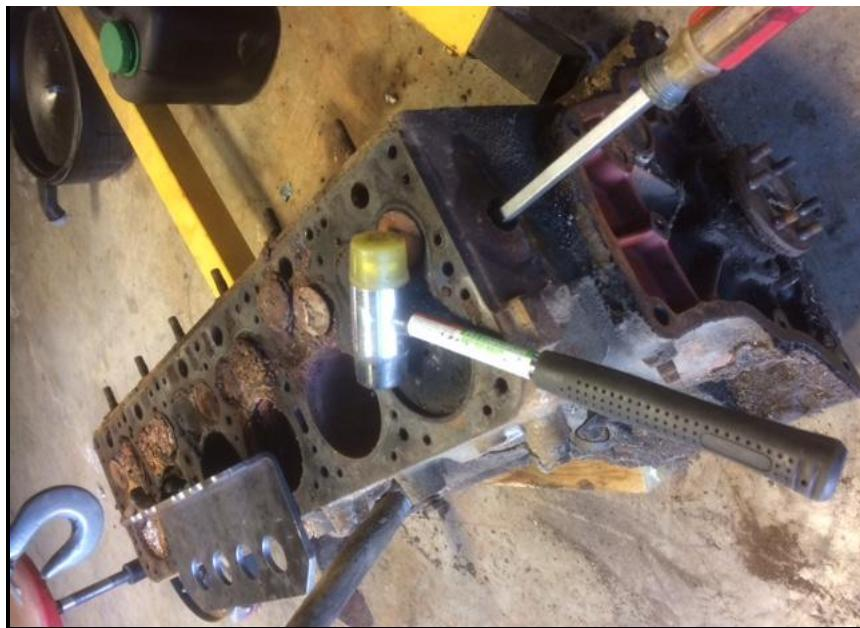
Step 5--- Both you and your assistant working together, using care will assure the tube removal with no or minimal damage. In case of large quantities of rust around the tube; working the tube slowly with lots of penetration oil to lubricate should overcome the rust.
