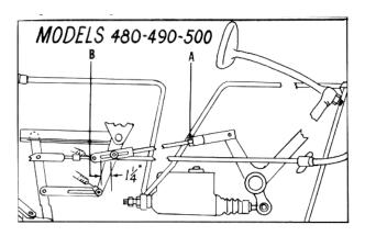
It will be noted that the adjustment for mechanical brake engagement shown in the sketches above differs somewhat due mainly to the change in design of various models. Adjust at "A" to obtain clearance at "B".
